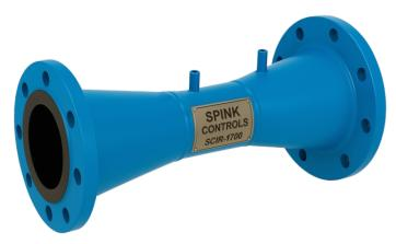
Spink Controls' Venturi Flowmeter is a highperformance differential pressure flow element designed for accurate measurement of liquids, gases, and steam. It operates on Bernoulli's principle, offering excellent accuracy with low permanent pressure loss and long-term stability. The smooth converging and diverging sections minimize turbulence and wear, making it ideal for large pipeline applications in power
