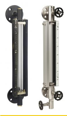
Gauge is fitted between two end fittings through gland packing. The gauge is mounted parallel to tank so as to form a close loop causing tank liquid to seek its level in the gauge. The Gauge Glass is protected with 'C' channel. End fitting has built-in isolating valve, drain valve & vent plug.
