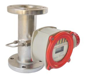
Spink Controls DP-based Gas Flowmeter is specifically designed to measure the flow of clean gases that are noncorrosive to silicon. The differential pressure ( $\Delta P$ ) is measured using a high-precision piezoresistive pressure-sensing element, where the applied pressure is converted into a differential voltage signal, approximately proportional to the pressure:  $V_{C}$   $\alpha \Delta P$
